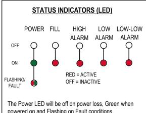
powered on and Flashing on Fault conditions.
