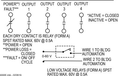
COLORED FROM POWER SUPPLY: **WIRE PAIR** 110VAC 110VAC **NEUTRAL** LINE OUT HIGH VOLTAGE VALVE WIRE 2 VALVE WIRE 1 POWER RELAY (LOAD) (LOAD) (FORM C) SPDT RATED MAX. 120V @ 40A
