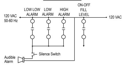
TO LOADS 120 VAC, 30 AMP, MAX. LOADS CAN BE VALVES, AUDIBLE OR VISUAL ALARMS
