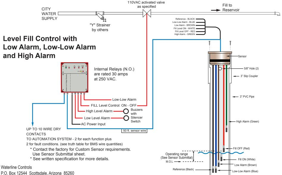
The 3" PVC Pipe needs to be at least 2" longer than the longest Sensor tip.
