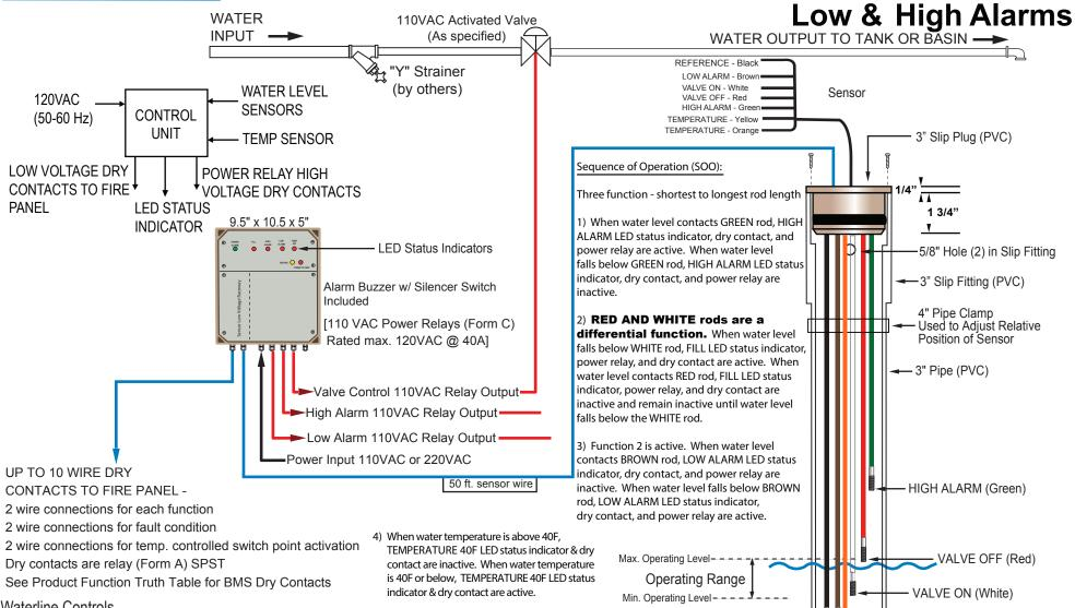
1. 3" PVC pipe of length greater than or equal to length of longest rod
