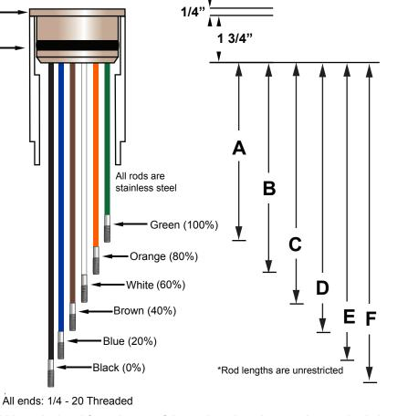
\*Dimensions should be calculated from the top of the tank or riser down to the required alarm level(s) in inches. Be sure to take into account any riser pipes or manway risers.
