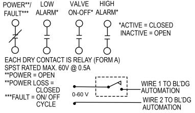
LOW VOLTAGE RELAYS (FORM A) SPST RATED MAX. 60V @ 0.5A
