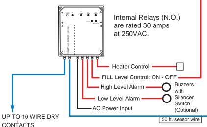
TO AUTOMATION SYSTEM - 2 for each function plus 2 for fault conditions. (see truth table for BAS wire quantities)
